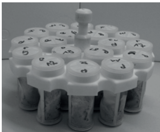
Fig. 1: Removal of soluble- (NDF), hemicellulose- (ADF), and cellulose- (ADL) fractions from the sample by heat, enzymatic and acid treatment, and filtration through Fiber Caps (FOSS, Germany)
